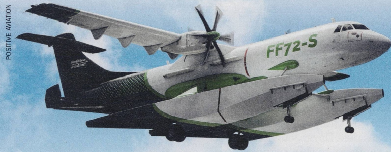
Positive Aviation plans to convert an ATR 72-200 into a float-equipped demonstrator this year.
